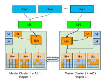
Fig.3 Large scale OLTP reference architecture - Master-Master Cluster in different Region via bi-directional synchronization
